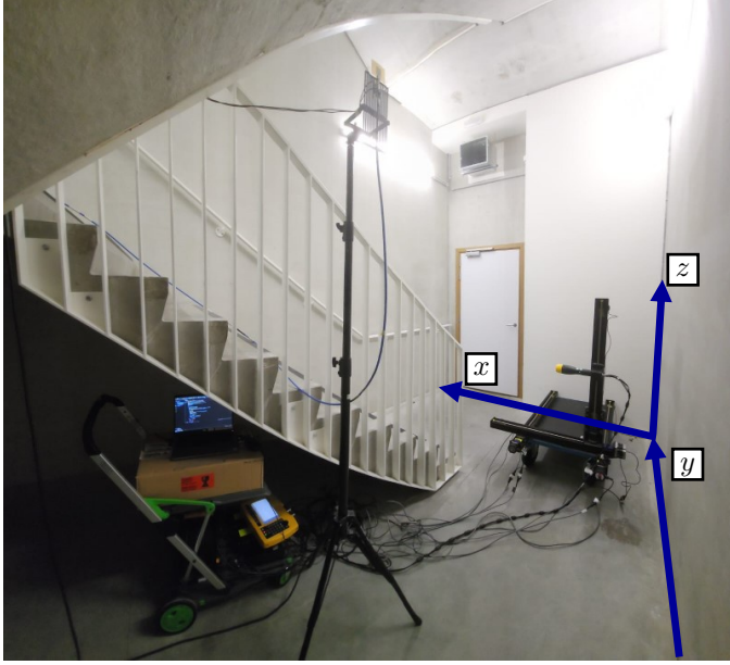
Fig. 1: Wide-angle photograph of the measurement setup. The robot (right) holds the Narda probe (yellow) and moves along the three cartesian directions: x towards the door, y normal to the right wall and z normal to the floor. The antenna (top, center) faces the right wall and radiates toward the setup at an angle.
